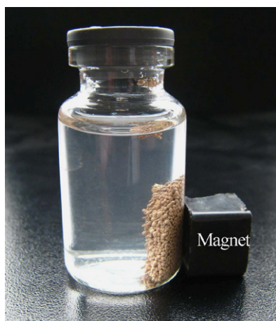
Fig. 4. Photograph of TBP/Fe 3 O 4 @PSF microcapsules attracted by a conventional magnet.
